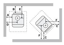
NOTE: Be aware that local Codes and Regulations may override some clearances listed in this manual. Check with your local inspector. Clearances to combustibles are for the safety of the property. To avoid overheating and damaging the appliance these clearances should be maintained for non-combustibles also.
