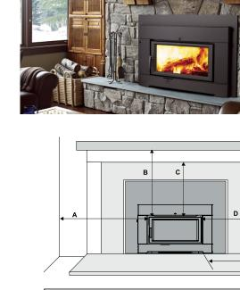
Minimum Hearth Extension for the front (E) and sides (F) are measured from the fuel door opening.
